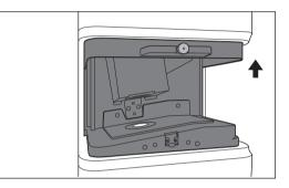
2 Install the transmittance zero calibration plate in a position so that it completely covers the illumination window.
